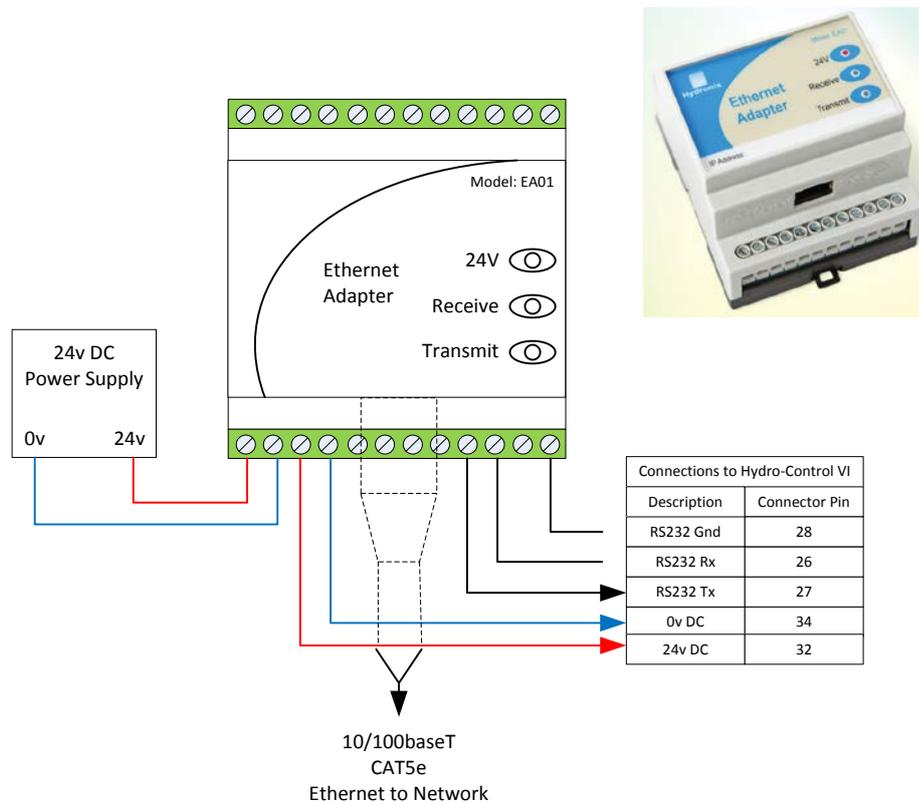
**Figure 5: Connecting the Ethernet Adapter to Hydro-Control VI**
