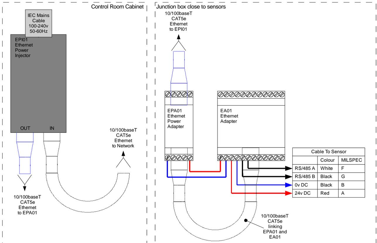
Figure 3: Connections for Ethernet Adapter and Power Adapter
