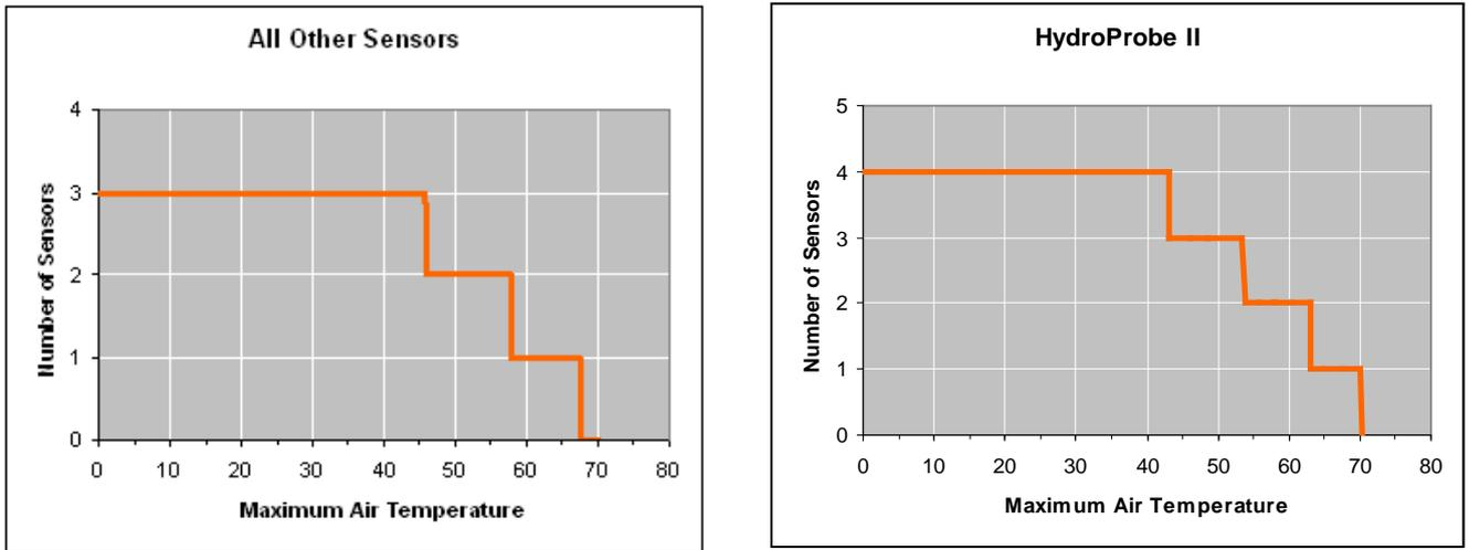
Figure 4: Maximum number of sensor connections dependent upon ambient temperature
